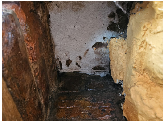
(Fig 4. Material taken from the edging of a fireplace; fibres can be seen within the sample taken)
