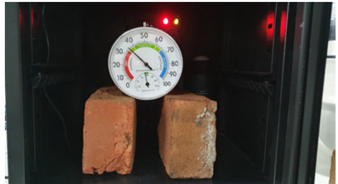
Figure 19: Farmhouse sample in electronically controlled desiccant chamber
